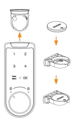
The Guub lock uses a CR2032 3V button cell battery which is rated for one year of normal use. The Guub lock will make three short beeps after being unlocked to warn that the battery needs replacing.
