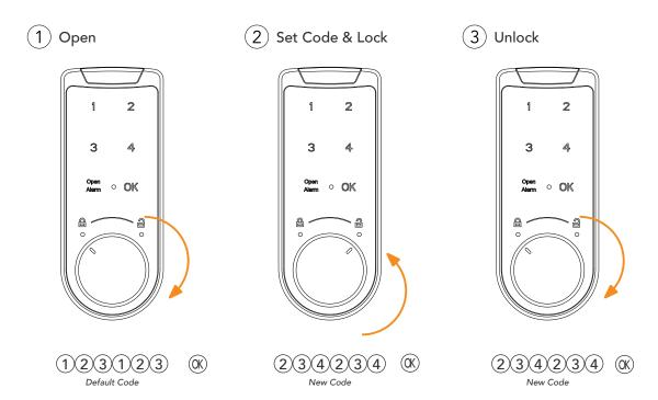
Public Mode is one-time password, where user code will be overrided after unlocking. Suitable for use when a locker will be used only temporarily by a user, setting their own combination to lock the locker for the day.
